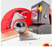
**RED** TM 300 is a programmable standalone machine for wire and wire harness taping. It features state of the art components that guarantee high level of precision and safety.
