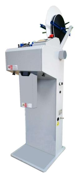
TC 7.0 is an electropneumatic hot cutting machine. It can cut a wide range of materials, with neat and precise results.
